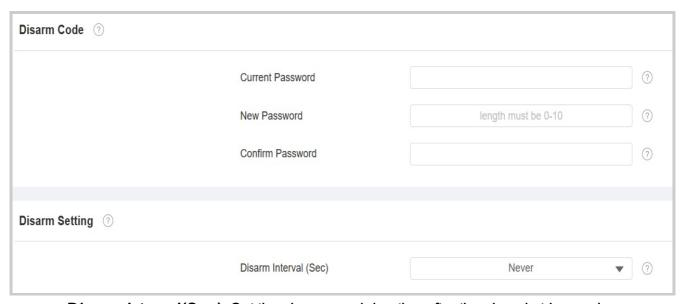
• Disarm Interval(Sec): Set the alarm sound duration after the alarm is triggered.
