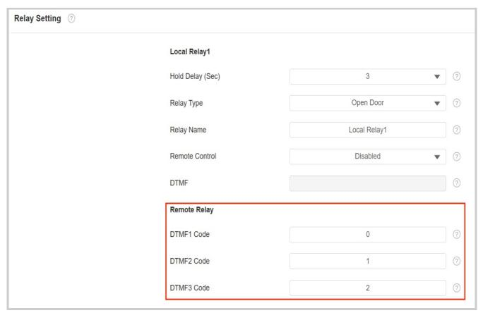
• DTMF Code: Define the DTMF code within the range(0-9 and \*,#) for the remote relay.
