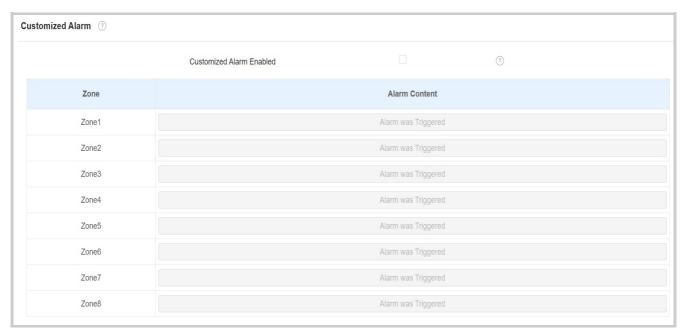
Alarm Content: The alarm text will display on the device screen when an arming is triggered.
