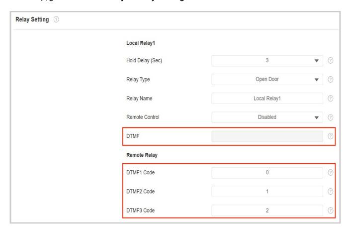
To configure the DTMF code transport format, navigate to the web **Account > Advanced > DTMF** interface.
