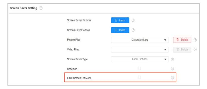
Fake Screen Off Mode: When enabled, the screen will turn off without a screen saver. The screen-saver parameters will be hidden on the web interface and the device. Third-party apps will keep running.
